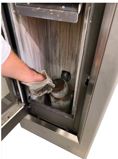
Fig. 32 - Burning pot extraction
