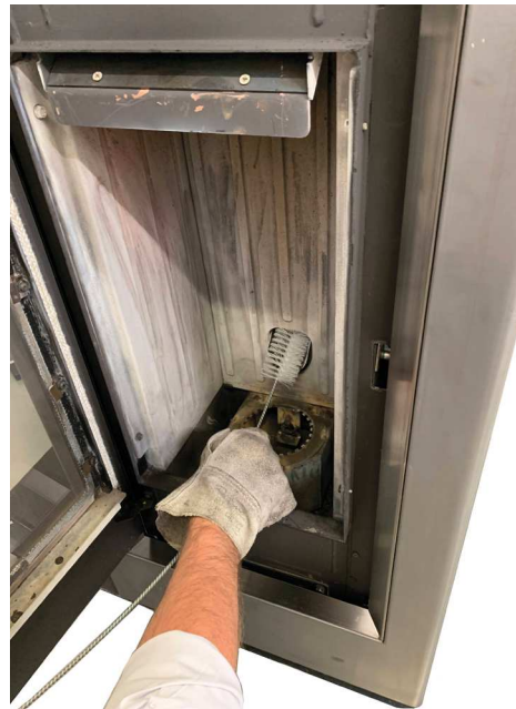
Fig. 39 - Cleaning with a brush
