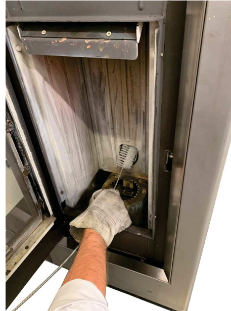
Fig. 35 - Cleaning with a brush
