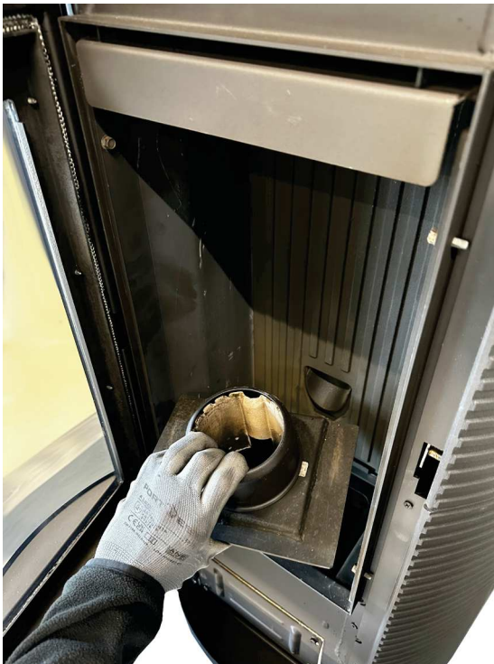
Fig. 36 - Burning pot extraction
