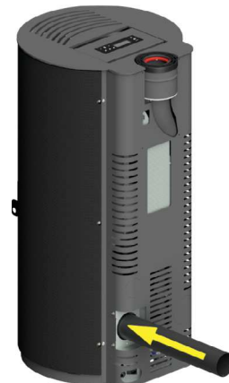
Fig. 50 - Connect the flexible
