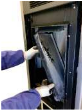
Fig. 75 - Remove the side walls
