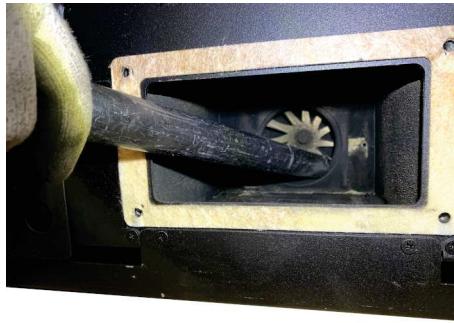
Fig. 82 - Vacuum out the ash
