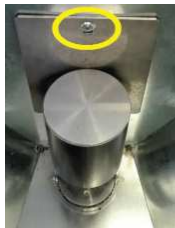
Fig. 91 - Remove the screw
