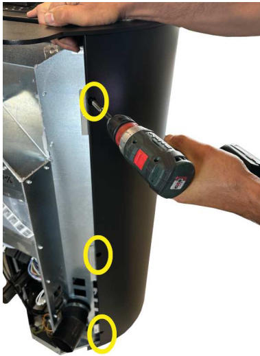
Fig. 25 - Remove the screws
