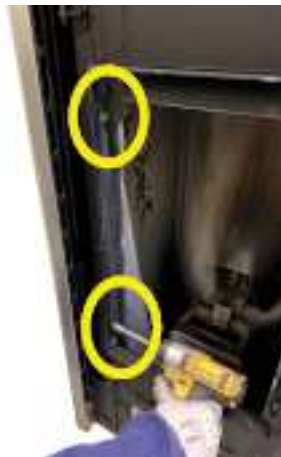
Fig. 72 - Remove the hex screws
