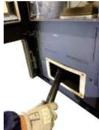
Fig. 78 - Vacuum out the ash
