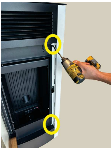
Fig. 34 - Remove the screws
