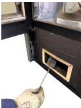
Fig. 68 - Clean with pipe cleaner
