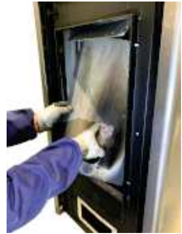
Fig. 76 - Remove the back panel of the firebox
