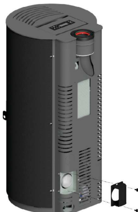
Fig. 49 - Remove the air diverter
