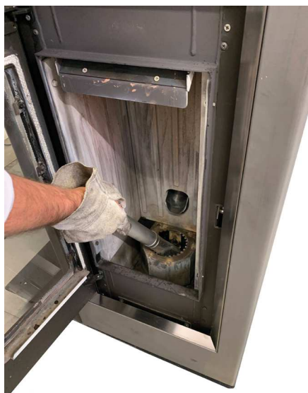
Fig. 36 - Burning pot box cleaning
