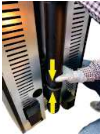
Fig. 58 - Connect the pipes
