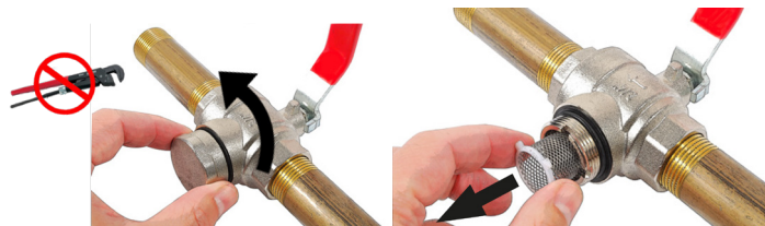
Fig. 7 - taking out the strainer
