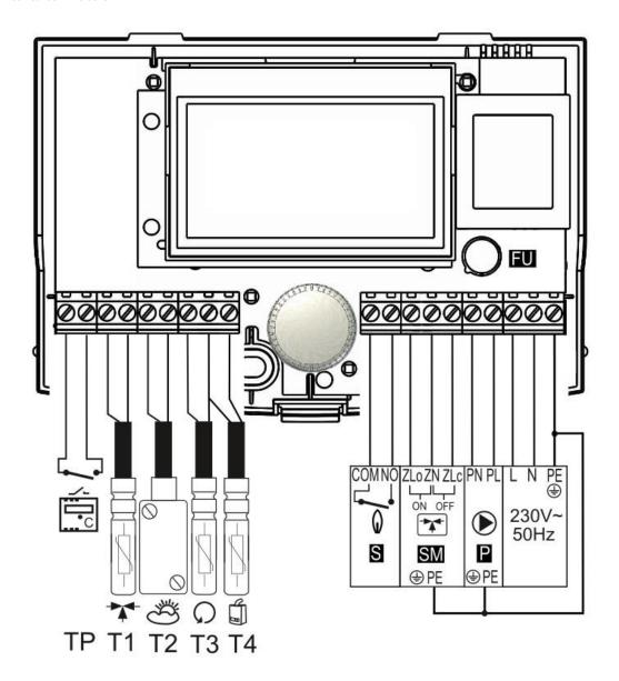
TP – room thermostat (No-Nc), T1 – temperature sensor mixer heating circuit type CT10, T2 – external temperature sensor type CT6-P, T3 – return temperature sensor type CT10, T4 – heat source temperature sensor type CT10, L N PE – power supply  $230V\sim$ , 50Hz, P – CH pump, SM – mixer actuator, S – contact to operate the heating source type 0N-0FF, FU – time-delay subminiature fuse.
