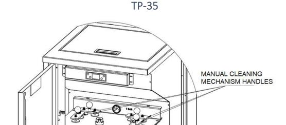
For the cleaning of the flame transmission pipes, manual cleaning mexhanism handles will be used. These handles are placed under the top plate for TP-16, TP-24, TP-30 AND TP-25 models, also placed inside the top cover for TP-35 model. Cleaning frequency must be daily and by removing the handles for 4-5 times.
