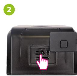
Make sure the camera is powered on. Then press and hold the button on the back of the camera for approximately 5 seconds, until the beep. The blue LED on the front of the unit will then start flashing. The pairing mode is enabled.
