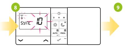
The thermostat started to send a signal to find the receiver (the symbol of the blinking antenna) and started the countdown with the number 10 (min). The pairing process may take up to 10 minutes.
