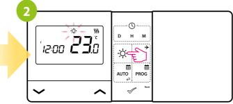
Press 🔅 button to enter comfort temperature mode. The sun icon should be visible on the display.
