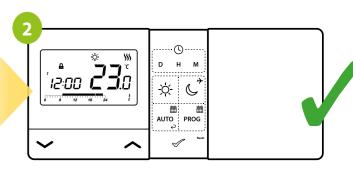
A lock icon will appear on the screen. The buttons on the thermostat have been locked.
