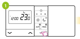
Check that the thermostat is not sending a signal to heat. Press any button to highlight the display.
