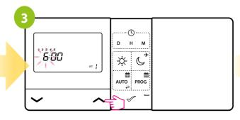
Using or buttons set the hour for the time period and then confirm by ✓ button.
