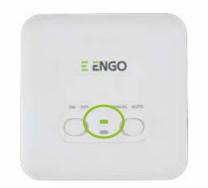
When the green diode on the receiver lights up continuously, the devices have been paired on a new frequency.
