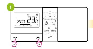
Press and hold  $\wedge$  and  $\checkmark$  buttons for 3 seconds.
