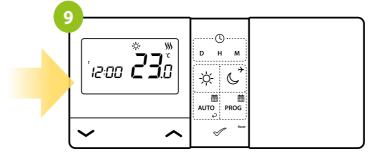
Set the temperature setpoint a few degrees lower than the room temperature by repeating steps 1 to 5. Wait a few seconds. The flames icon should stop animating...
