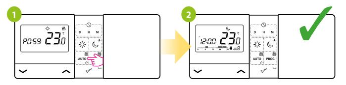
To cancel the function, press any button to turn on backlight and then press 2 times AUTO button.
