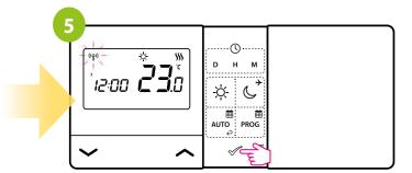
The thermostat started sending a heating signal when the screen went blank, which was signaled by the antenna symbol.
