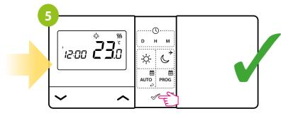
The thermostat will return to the main screen and display the actual room temperature.
