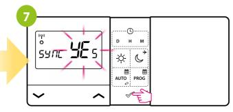
Using or buttons choose YES and start the pairing process on a new frequency by pressing the button.
