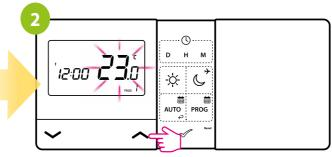
Using **∼** or **∨** buttons set temperature setpoint during active AUTO mode.
