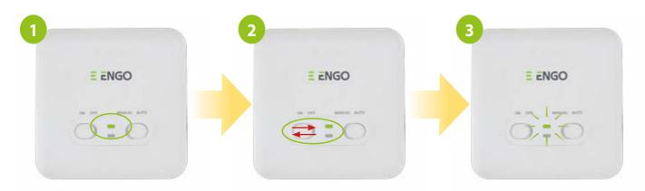
If you want to re-pair the devices with each other, make sure that the receiver is disconnected from the power supply and the switches on it are in the AUTO and ON positions. Then connect the receiver to the power supply and wait for the green diode to glow continuously.
