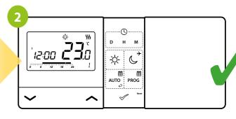
The lock icon will disappear from the screen. The buttons on the thermostat have been unlocked.
