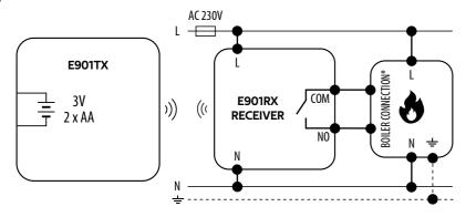
b) Connection diagram to the pump / actuator
