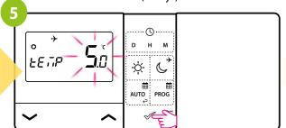
Use **∼** or **∨** buttons to set temperature setpoint which thermostat will maintain for defined number of days. Confirm by  $\checkmark$  button.
