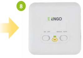
Check that the orange LED on the receiver is on. If so, it means that the communication between the devices is correct.
