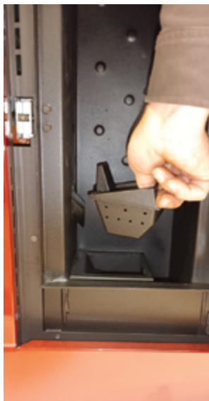
Fig. 32 - Burning pot extraction
