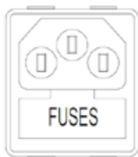
Fig. 37 - Shutter with fuses to remove
