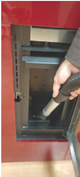
Fig. 34 - Burning pot box cleaning
