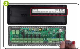
Connect the wires in accordance with the connection description.
