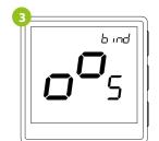
Release the keys, binding function process of linking thermostat with control box is active.
