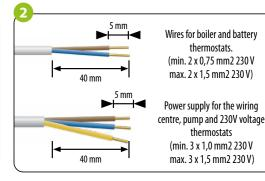
Remove the appropriate piece of insulation from the wires
