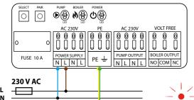
Power supply for wiring centre is  $230 \text{ V} \sim 50 \text{Hz}$ .
