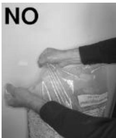
*Fig. 24 - Wrong opening of the pellets bag*
