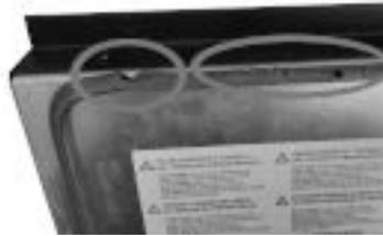
Fig. 27 - deteriorated gasket
