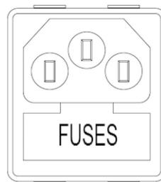
*Fig. 35 - Shutter with fuses to remove*
