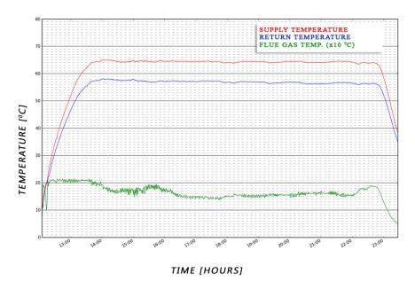
and the controller without PID control:
