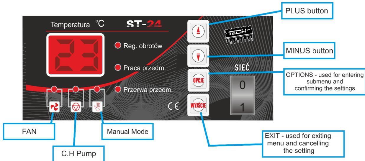
Microprocessor-based ST-24 Sigma regulator is intended for controlling CH boilers equipped with blow and CH pump. Its main task is to maintain the pre-set temperature with the use of a fan.
