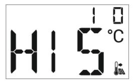
When the floor temperature reaches 33°C, the underfloor heating will be disabled. It will be activated again when the temperature drops to 31°C.
