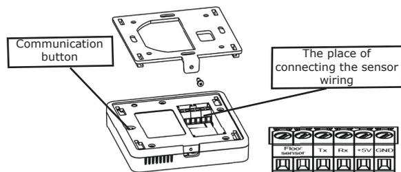
Mount the EU-R-9z sensor hanger on the wall and next fit the cover.
