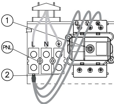
*PNL - connection points of neutral, protective, and phase conductors*
