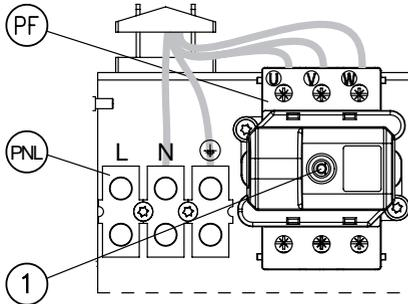
*PNL - points of neutral and protective conductor connection*
