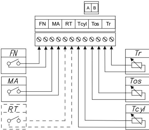
*FN - external adjustment of selected room temperature*
